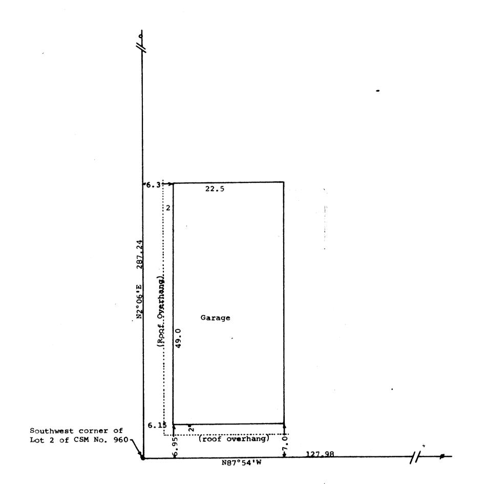
Scale - 1" = 10° •= 2" Iron Pipe Found #= 3/4" Iron Pipe Found o = Iron Pipe Found - Size not noted Bearings shown are those of record on CSM No.
